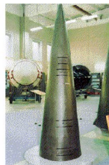
200 kt thermonuclear warhead deployed from 1981 to 1991 for a 450 km range operational-tactical missile which was withdrawn from service under the INF Treaty, in exchange for the American Pershing INF disarmament.
